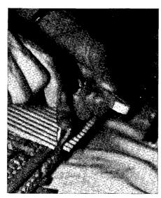
1. Hammers are reamed with a tapered reamer from the front side.
